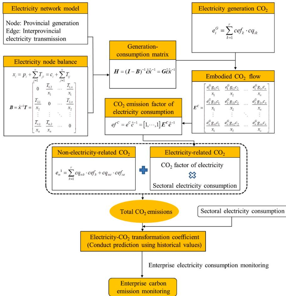
Fig. 1. Framework of enterprise carbon emission monitoring using electricity big data.
