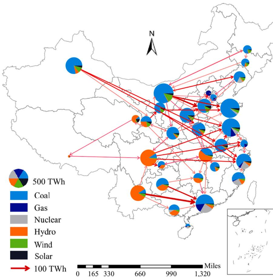
Fig. 3. Electricity generation structure and interprovincial electricity transmissions in 2020.
