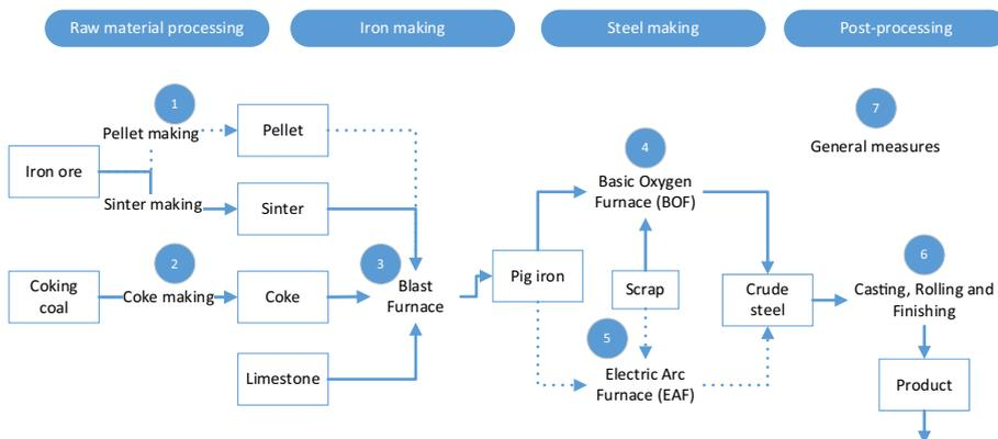
**Fig. 1** Schematic flowchart of iron and steel production and the seven key energy-intensive processes
